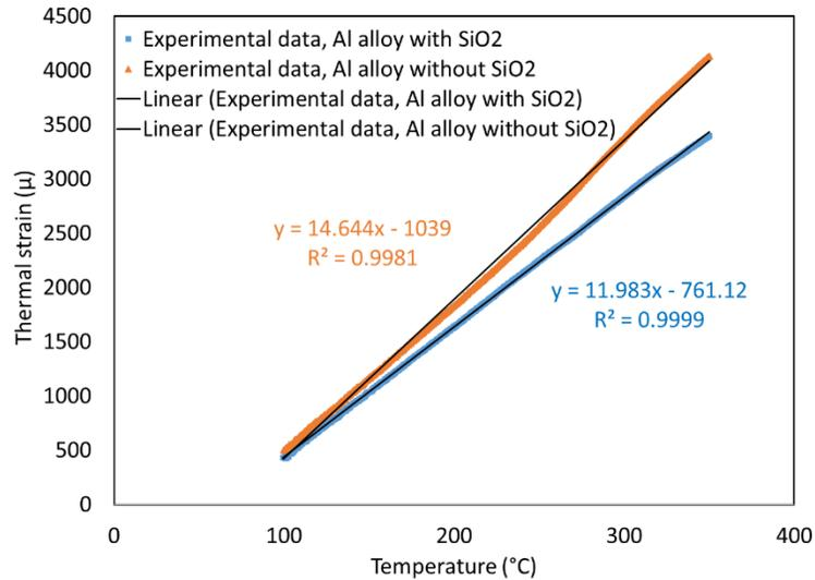
**FIGURE 4.** Results of dilatometric measuring for aluminum alloys, (a) without and (b) with nano-particles.
