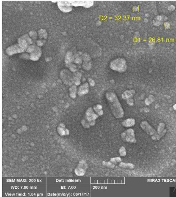
FIGURE 2. The FE-SEM image for the distribution of nano-particles in the matrix.
