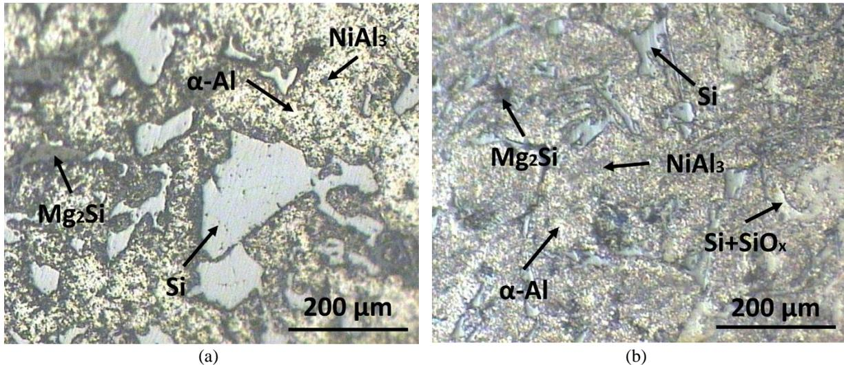
FIGURE 3. The microstructure of aluminum alloys, (a) without and (b) with nano-particles, by the optical microscopy.
