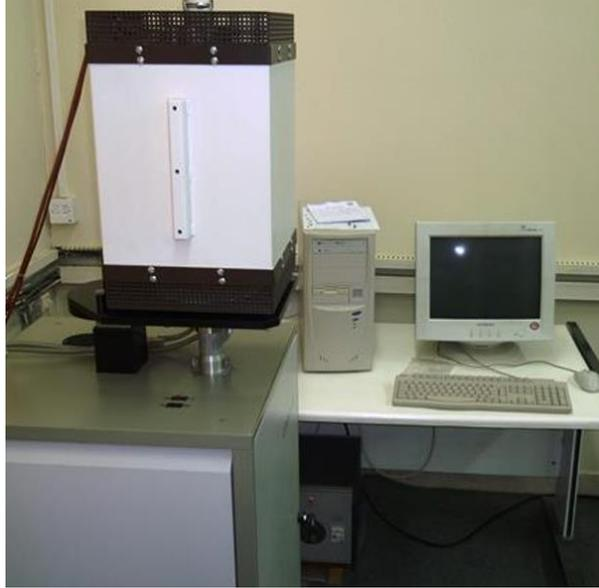
**FIGURE 1.** The dilatometric equipment for the analysis of thermal properties.
